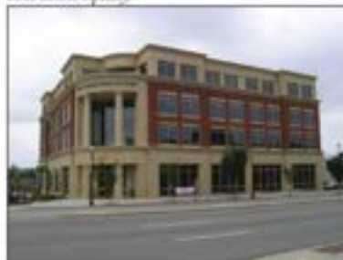
Good example of appropriate corner treatment for a corner building with two primary street frontages. The rounded corner and change in color distinguish the entry from the rest of the building.
