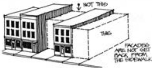
Figure 2.1.1 New, infill buildings should be set approximately the same distance from the road as adjacent buildings.
