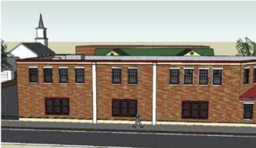
The placement of the windows both horizontally and vertically reinforces the bays with a slight modification in the pattern between bays. The windows are also aligned vertically and horizontally. The windows are approximately six feet in height and the building façade is approximately 20 feet in height. Notice also that the distance between the top and bottom row of windows is not greater than the height of the windows.
