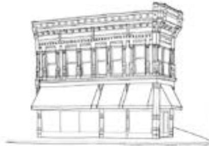
Illustrations depicting appropriate and inappropriate placement of awnings. Awnings at top do not respect the supporting frame of the building nor the corner entrance. Awnings at bottom fit within the building frame and break at the corner to highlight entry.
