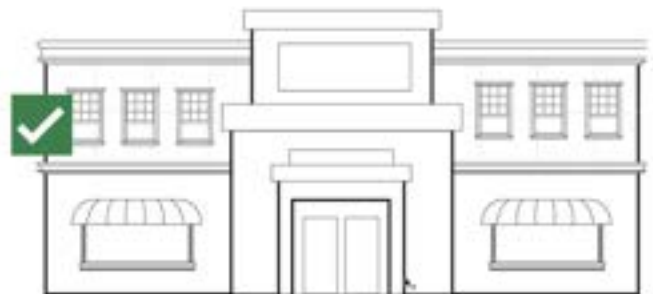
The three elevations show the same size building façade of about 20 feet in height. The first image is unacceptable because it appears very boxy and out of character with the Neighborhood Areas. The acceptable options show how the same size façade can be modified to appear as if it is a two-story building and break-up the mass of the structure.
