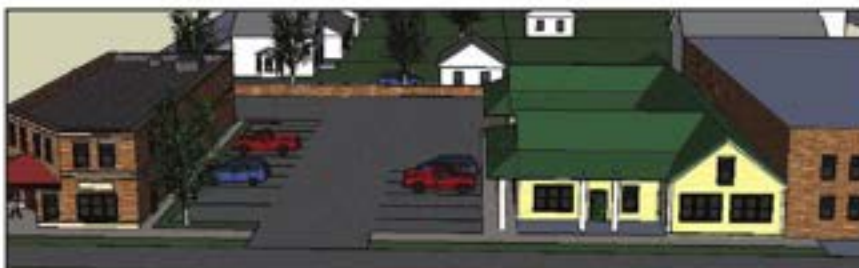
Some visible parking to the side of Commercial-Type buildings is permissible. This illustration shows a parking area approximately 80 feet in width. To maintain the building rhythm no more than 80 feet of continuous frontage along a block should be dedicated to surface parking.
