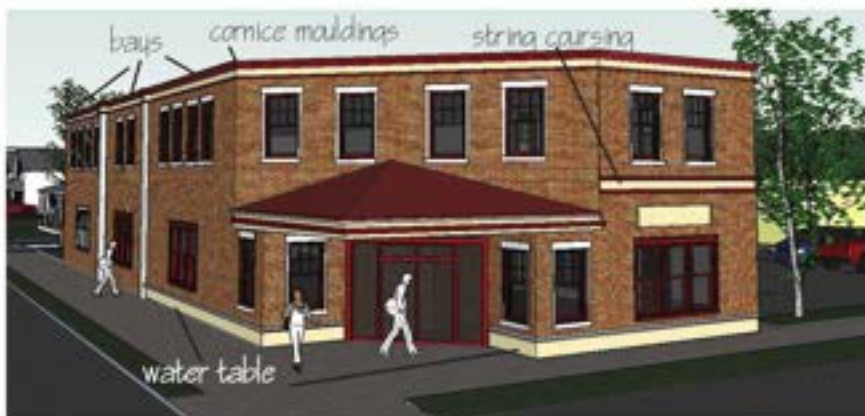
The longer façade of this building is articulated both vertically and horizontally through the use of bays and a water table, string coursing and a cornice moulding.
