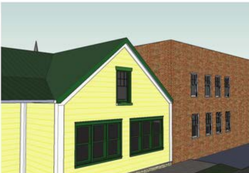
Although these two buildings are different styles and have different windows, the windows are aligned vertically along the block creating consistency and reinforcing a unified character for the area.
