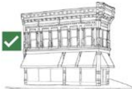
Figure 3.11.1 Illustrations depicting appropriate and inappropriate placement of awnings. Awnings at top do not respect the supporting frame of the building nor the corner entrance. Awnings at bottom fit within the building frame and break at the corner to highlight entry.
