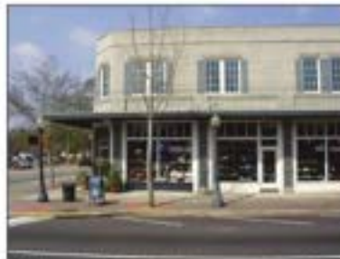
Good example of appropriate corner treatment for a corner building with two primary street frontages. The 45 degree corner allows the entry to address both streets equally.
