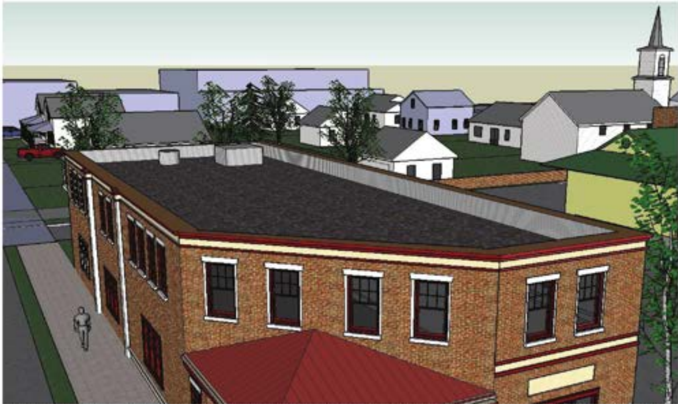
The use of a parapet and dimensional cornice moldings adds depth and character to the building. Additionally the parapet serves as an integrated element of the building that screens roof-top equipment.
