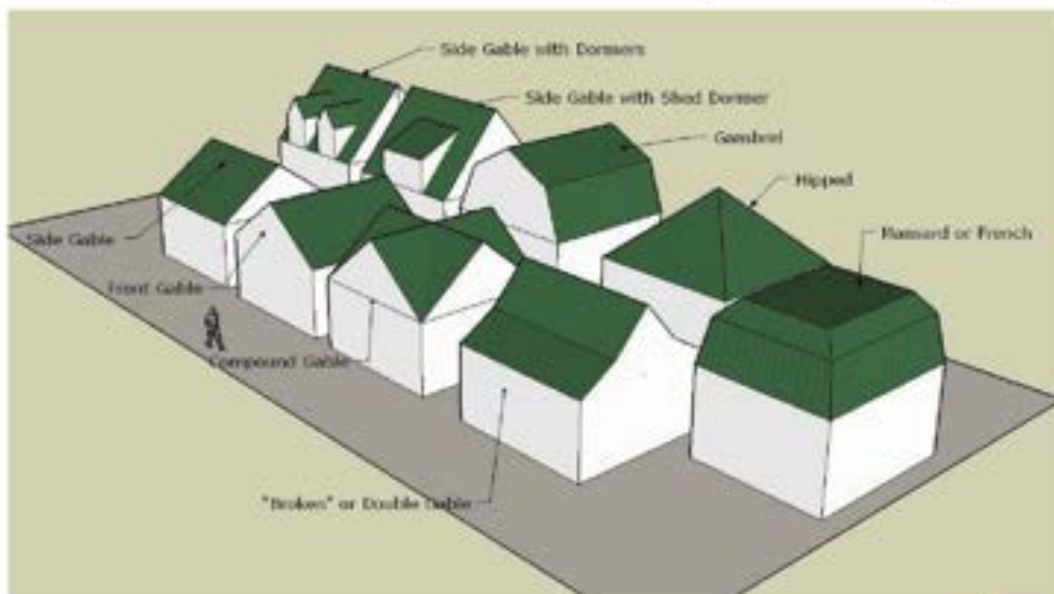
The illustration to the left shows the different types of pitched roof forms, most of which are appropriate on single-story buildings except the Mansard or French roof.
