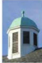
Traditional roof structures such as these cupolas can be used to house roof top equipment on gabled roof forms. On flat roofs with parapets, equipment can be placed out of site by keeping the parapet higher than the equipment.
