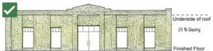
This illustration shows a building façade with 25% of the linear width dedicated to window and door openings. An adequate quantity of glazing on the primary façade is the most important, secondary façades do not need to have as much glazing.
