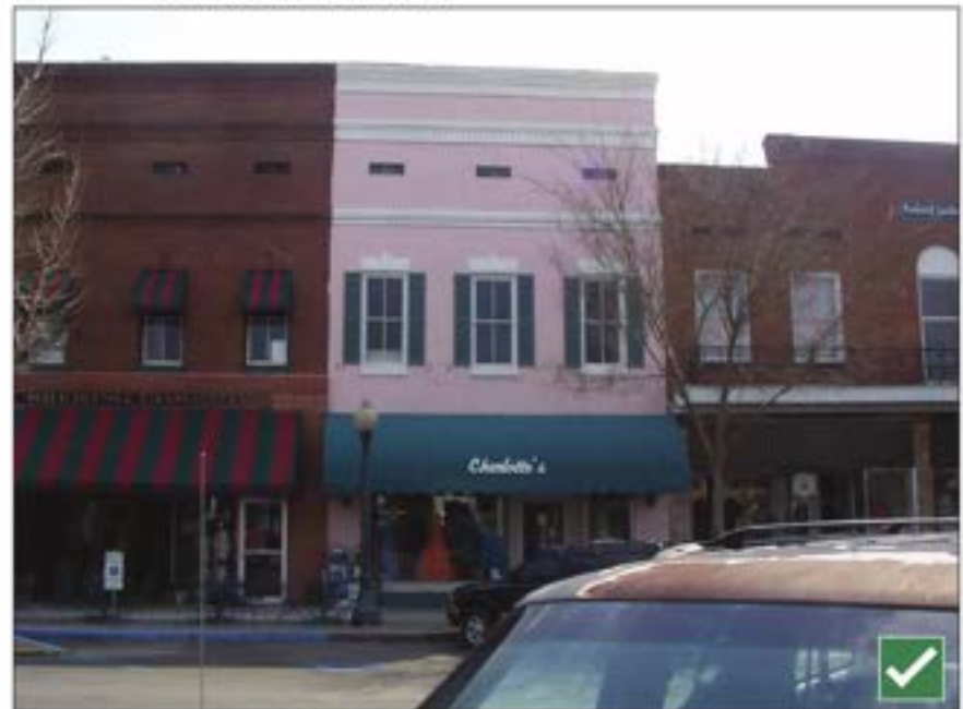
Disimilar buildings (in terms of style, color, etc.) are unified by the alignment of architectural elements such as awnings, canopies, storefront heights, etc.
