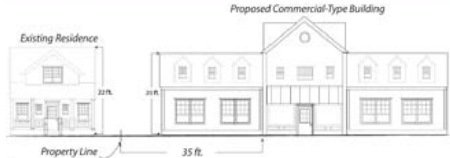
Above: A proposed commercial-type building should respect the adjacent residence by stepping up the building height over twenty feet only at a distance of 35 feet from the shared property line.
