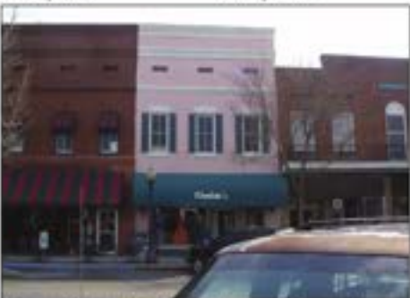
The consideration of horizontal alignment of door (storefront) and window elements unifies these three buildings of dissimilar heights, colors and detailing. Proportionality, however, is essential to a unified street.
