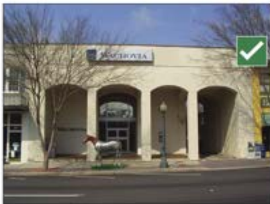
Good example of new construction that aligns with adjacent buildings. Recessed entry is utilized, yet columns maintain the alignment of the “street wall” created by the building faces.
