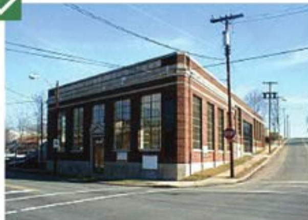
This historic industrial structure from Charlotte, NC illustrates how a tall single-story building can be appropriate when large-scale windows are used in conjunction with other architectural details. If this building did not have the tall windows it would seem much larger than it does because of the large surface planes that would be exposed.
