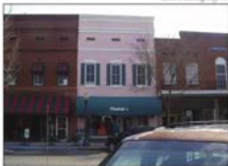
The consideration of horizontal alignment of windows unifies these three buildings of dissimilar heights, colors and detailing.
